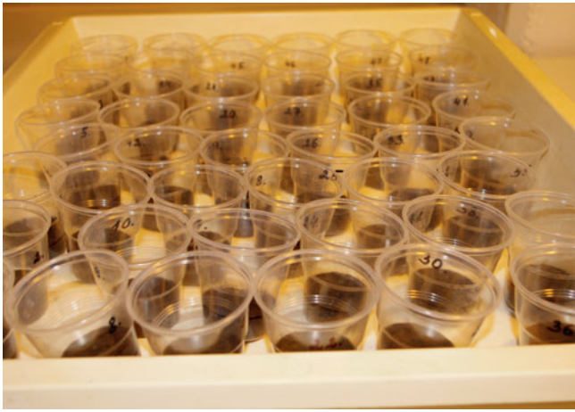
Figure 2 A set of 48 PVC beakers completely randomised on a plastic tray. Each sampling time corresponded to one tray.
