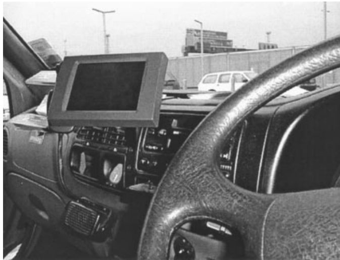
Figure 1. The touchscreen MDT installed on an RAC patrol vehicle.
