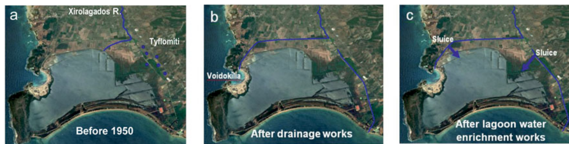
Figure 2 Changes in the lagoon hydromorphology during the last 70 years: (a) before 1950; (b) after attempts at lagoon drainage; (c) after the 1998 water enrichment works. The Tyflomiti springs are shown by blue dots and artificial sluices by blue arrows. (Personal communication with Hellenic Ornithological Society.)
