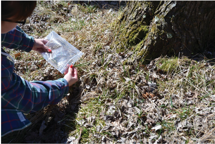
FIGURE 7. Vegetation collection. Care should be taken to collect only from one species of plant. Dead and dried samples are preferable. If live plants cannot be dried immediately, then the sample bag should be left open to allow for evaporation. Once back in the lab, remove from the bag to allow for complete drying.
