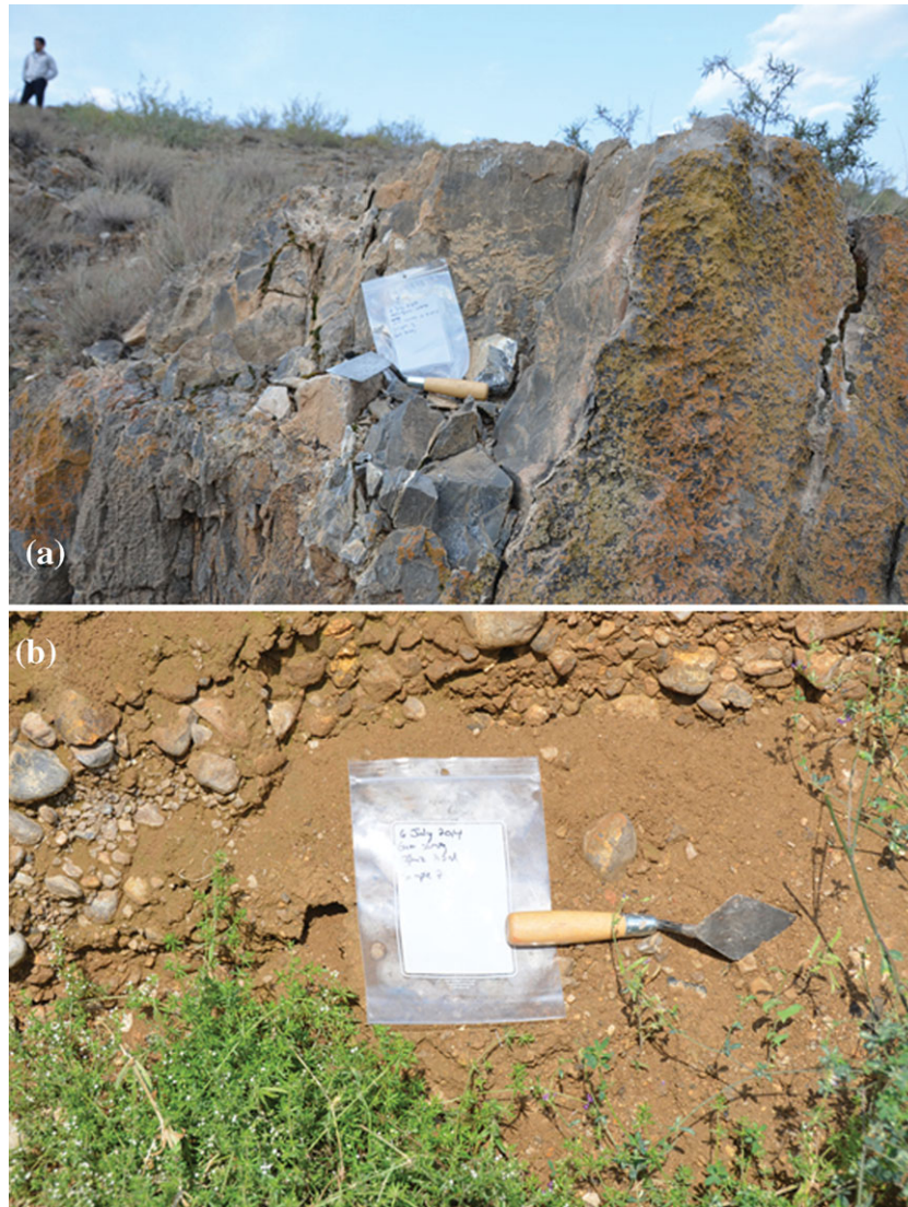
FIGURE 6. Rock and soil sample methods: (a) use a very small sample of rock for ^{87}\text{Sr}/^{86}\text{Sr} , which can be collected via 50 mL centrifuge tubes or standard field collection bags; use a rock hammer to expose and collect samples with fresh surfaces (i.e., not exposed to previous erosional processes); (b) collect soil samples in a 50 mL centrifuge tube or standard field collection bag; expose a fresh surface and collect at least 5 mg of soil.
