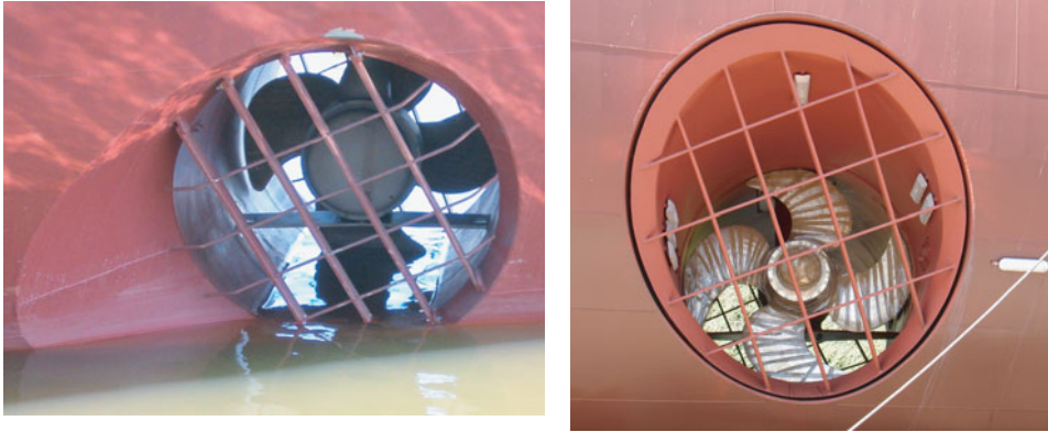
Figure 5. Left: A typical tunnel bow thruster with a protection grid and a conical fairing at the aft part (source http://en.wikipedia.org ). Right: A modern protection grid with a hull-thruster sharp transition (source: author).
