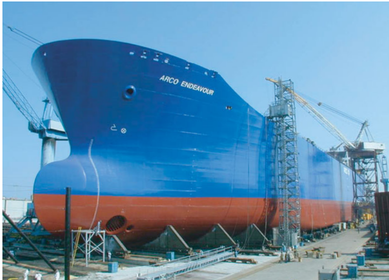
Figure 9. The tanker "Polar Endeavour" (ex "Arco Endeavour") showing the bow thruster with an AST (a 2207 kW thruster of 2.4 m diameter with a 0.8 m diameter AST). Photograph: author.
