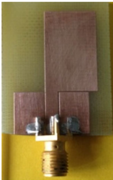
Fig. 8. Photograph of the fabricated FGCPW-fed flag-shaped UWB monopole antenna.
