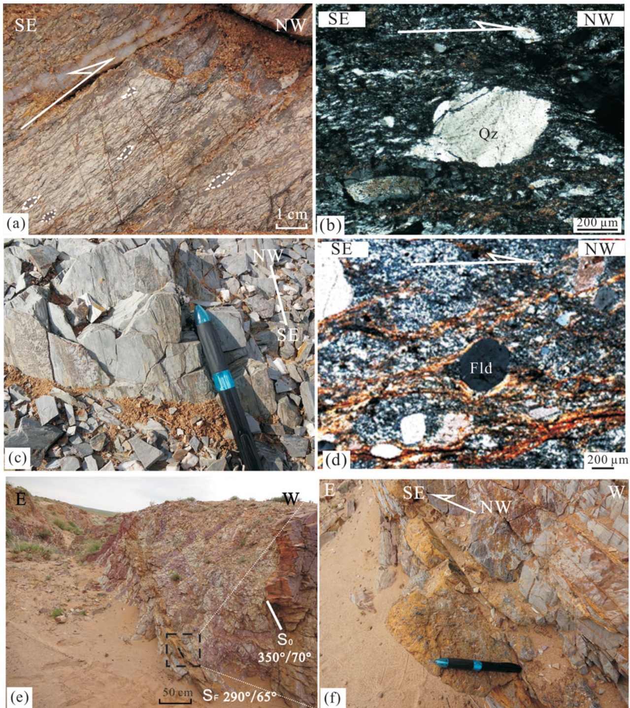
Figure 5. (Colour online) Photographs of NW- or SE-directed thrusts of the D2 stage of deformation in the Mandula area. (a) Mylonitic granites preserved in the F5 thrust faults (GPS: 42^{\circ}25'08''\text{N} , 110^{\circ}27'41''\text{E} ). (b) Microfabrics show a top-to-the-NW shearing; Qz – quartz. (c) Foliated marlstones (the Baotege Formation, Early Permian) along the F6 fault. (d) Sigmoidal porphyroblast of feldspar showing a top-to-the-NW sense of shear in the mylonitic sandstones of the F6 fault; Fld – feldspar. (e) SE-directed thrust (D2) cross-cuts the N-dipping turbidite (D1), found in the Lower to Middle Permian Dashizhai Formation; the fault plane ( S_F ) dips to the NW and the beds ( S_0 ) dip to N. (f) Fault breccias and mirror surface with pseudotachylite are observed close to the fault. Length of pen for scale is 15 cm.
