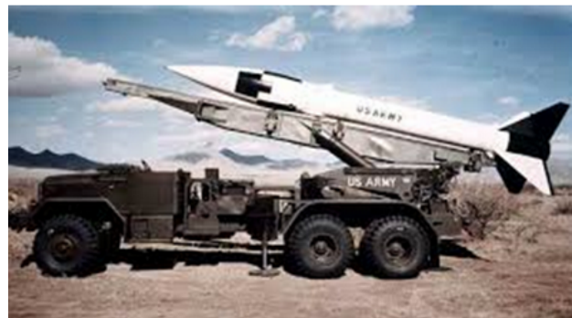
Nuclear-capable Honest John rocket on its truck-transported launcher.
