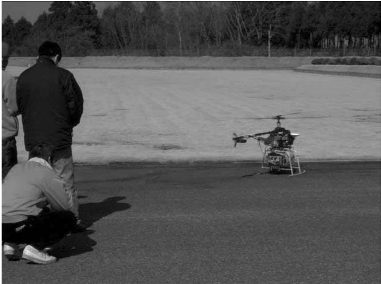
Fig. 1. Small-scale unmanned helicopter (SF-40).
