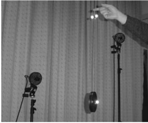
Fig. 1. Measurement of yo-yo motion with optical system SMART.
