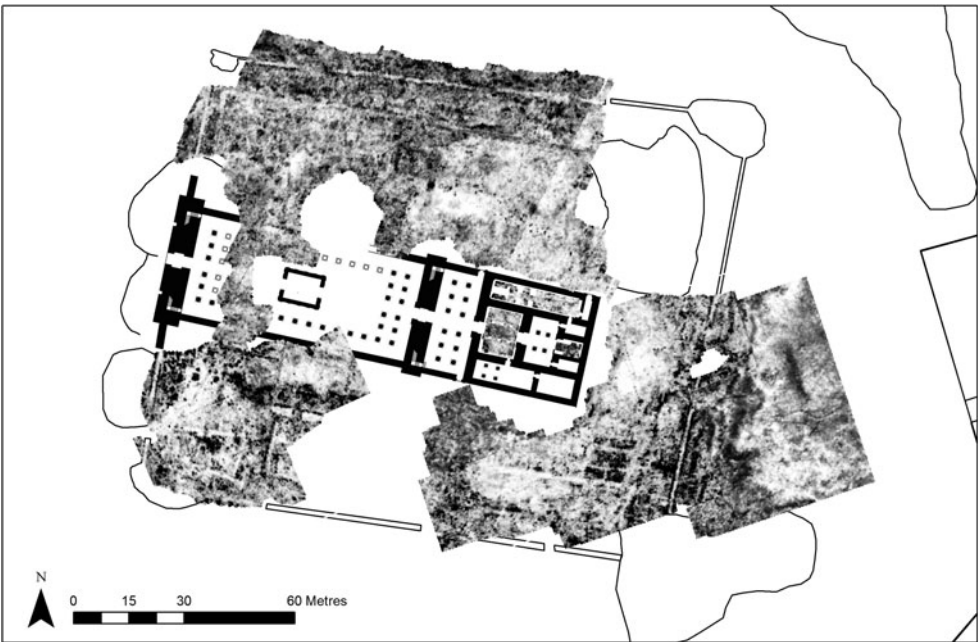
Fig. 2. Dangeil, Sudan. GPR survey results within the sacred precinct showing the main architectural features. (Plan of temple: J. Dobrowolski.)
