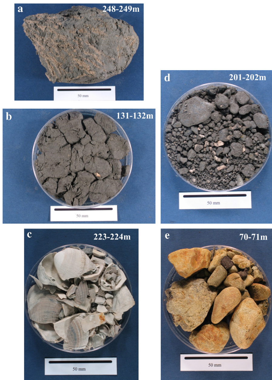
Figure 3. Photographs of a range of units identified within the hole; a) blue-grey fossiliferous mud of facies M containing siliceous Polychaete tubes; b) mica rich unconsolidated silty sand from facies FZS; shelly gravel of c) facies SL and d) facies SG; and e) subangular–subrounded greywacke clasts of facies G.
