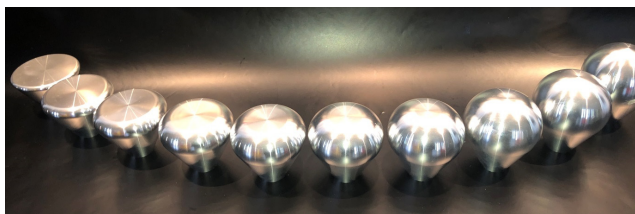
Figure 4. Wind tunnel models used to study the influence of the shoulder radius (transition from a 90^\circ cone to a sphere).
