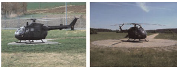
Fig. 3. BO 105 Helicopter without launcher (left) and with missile launchers (right) on turntable.
