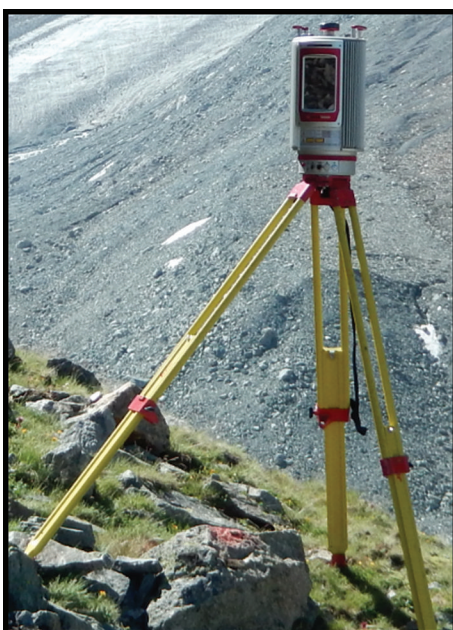
Fig. 2. Terrestrial laser scanner RIEGL VZ-6000 used for the surveys, in front of Haut Glacier d'Arolla.
