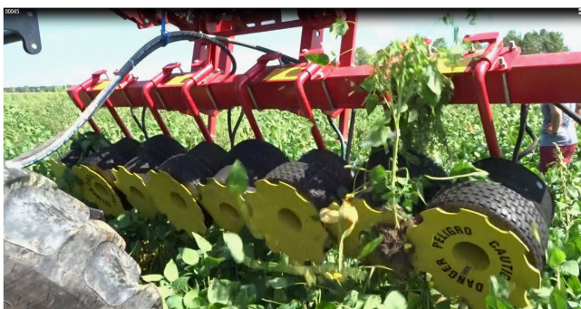
Figure 1. The Bourquin Organic Weed Puller® mounted on a tractor. The image is a screenshot of a video taken in soybean plots during the trial. A pulled, uprooted common lambsquarters is visible on the right.
