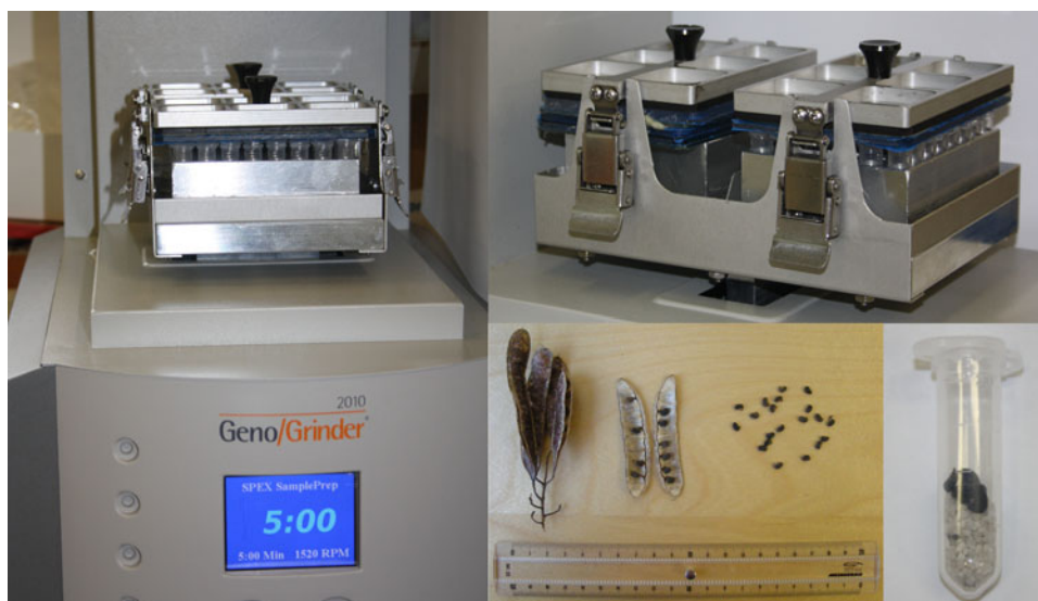
Figure 1. The grinder used to break seed dormancy. The seeds and sand in the tubes are shaken homogeneously controlling both speed and duration to quickly achieve a homogeneous sanding of the seed coat. On the right, close up of the plates allowing shaking of 96 tubes at a time, with a view of the pods and seeds as collected from the pods and in the tube ready for sanding (5 seeds per tube). Photograph credits: X.P. Bouteiller and A.J. Porté.
