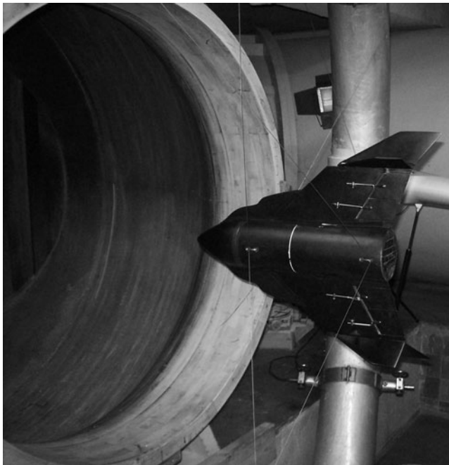
Figure 5. Experimental model of the Rocket Plane hung in the wind tunnel (configuration 1211).
