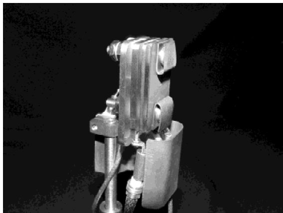
Fig. 5. Electrical connections to the Faraday cup, the faceplate, and the secondary electron suppression plate allow us to measure charge striking any surface. The copper shield prevents stray ions from impacting the wire leads.
