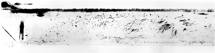
FIGURE 20. A section (110 mm \times 19.2 mm) of the upper part of the flow channel. Instead of ferrofluid it is filled with a suspension of tracer particles in water. The impressed flow velocity was U = (0.207 \pm 0.006) \text{ m s}^{-1} , the exposure time t_{exp} = 500 \text{ ms} . The black dashes mark streaks, indicating the propagation of the tracer particles during t_{exp} .
