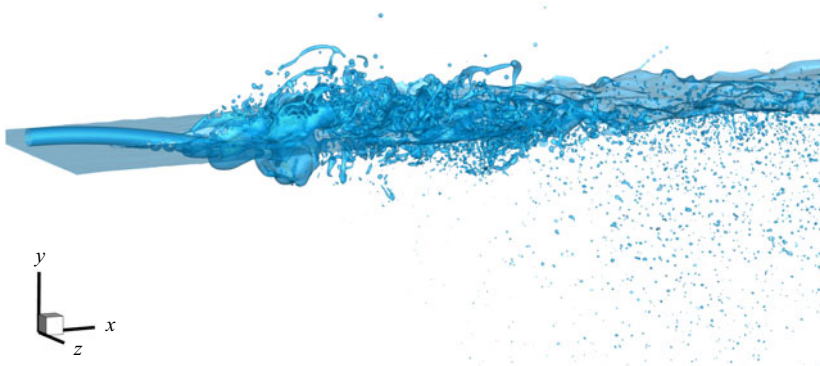
Figure 2. Simulation result of instantaneous air–water interface visualized using the iso-surface \phi = 0 . The result for case 6 is shown.
