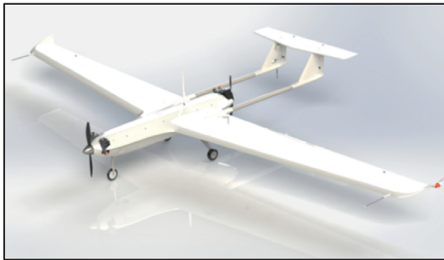
Figure 1. The UAS-S45 Balaam.
