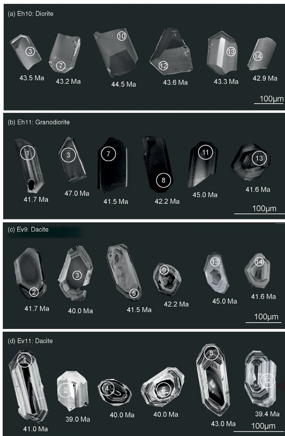
Fig. 6. (Colour online) Cathodoluminescence (CL) images for zircons from the magmatic rocks of the region south of Birjand. Circles indicate the position of laser spots for zircon U–Pb analyses. Analytical numbers and ^{206}\text{Pb}/^{238}\text{U} ages are also shown. Scale bars are 100 \mu\text{m} across.
