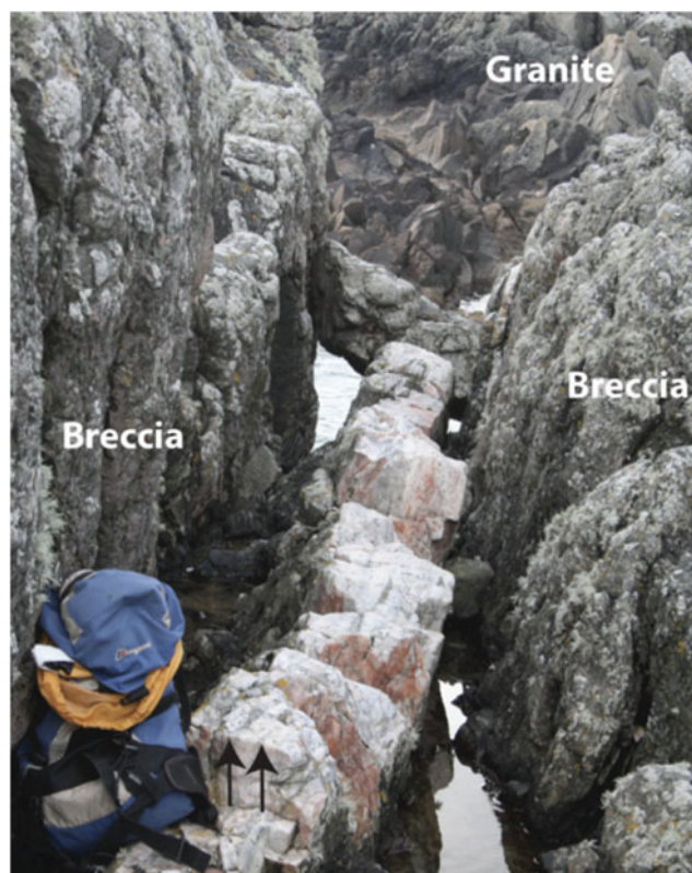
Figure 3 Field photograph showing the targeted quartz–molybdenite vein hosted by intrusive breccia (sample point 3 in Fig. 2). Non-xenolithic granite can be observed in the background. Black arrows show molybdenite- and muscovite-rich grey streaks through the vein.
