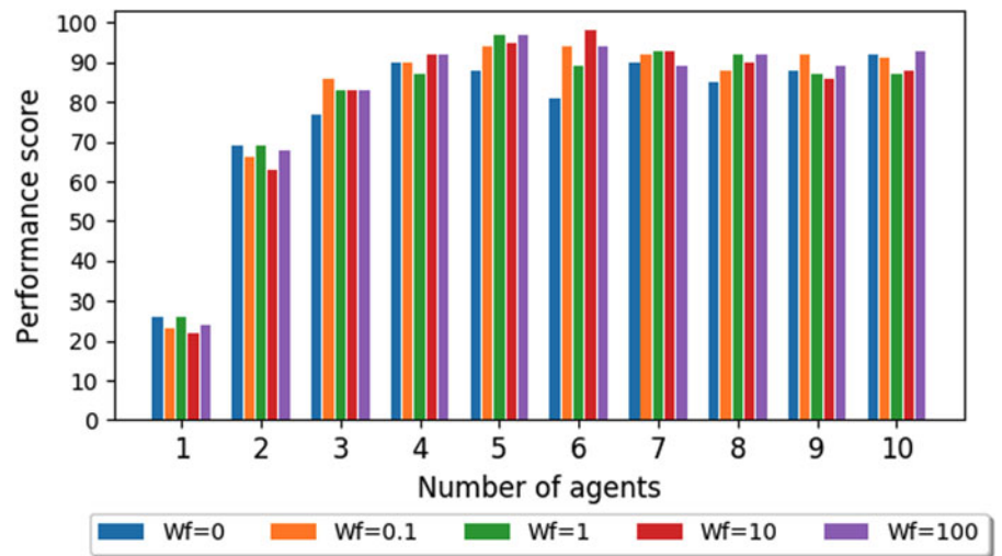
Fig. 8. Sensitivity of performance score with different weight factors of rotation reward in different number of agents in box-pushing task.
