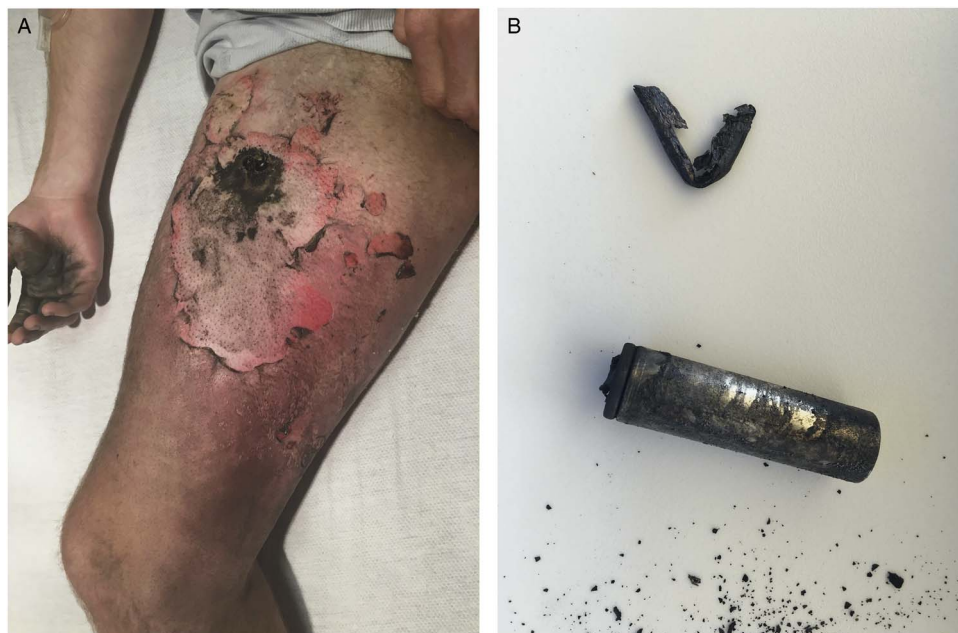
Figure 2. A) Anterior right thigh burn of the patient in Case II on the day of the burn injury. B) E-cigarette battery device and fragment of the casing removed from the thigh of the patient.
