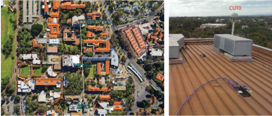
Figure 6. Observation conditions and GNSS antennae ( http://www.igs.org/images/site/CUT0_1.jpg ) used in zero and short baseline experiments at Curtin University Bentley campus.
