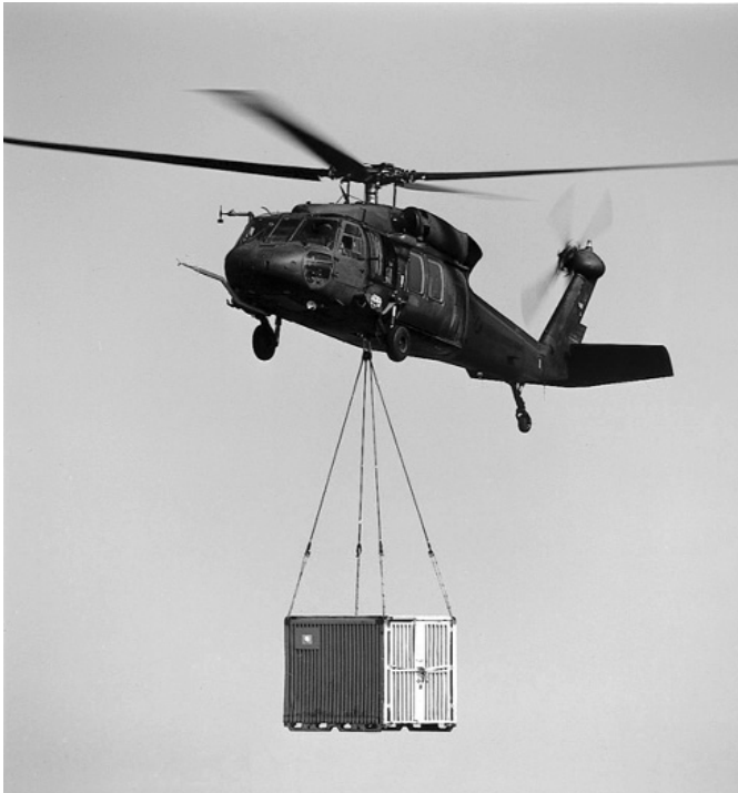
Figure 1. UH60 – CONEX slung load configuration.
