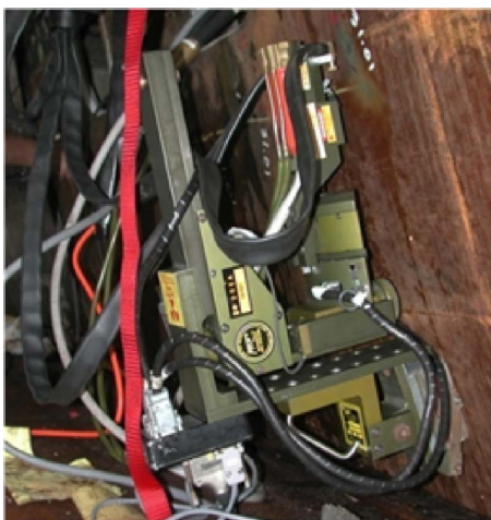
Figure 1. (Color online) The mXRD is shown during on-site measurement of residential stress on a submarine pressure hull. The mXRD goniometer is supported by the field stand that is attached to the submarine pressure hull using a large permanent magnet. The goniometer consists of the X-ray tube and beta rotation motors.
