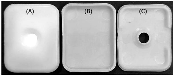
Fig. 1. The configuration of flow-through DIGFA device. (A) Whole device filled with water-absorbing pads and a porous nitrocellulose membrane coated with antibodies laid on the top; (B) support box; (C) box cover with a hole-opening.
