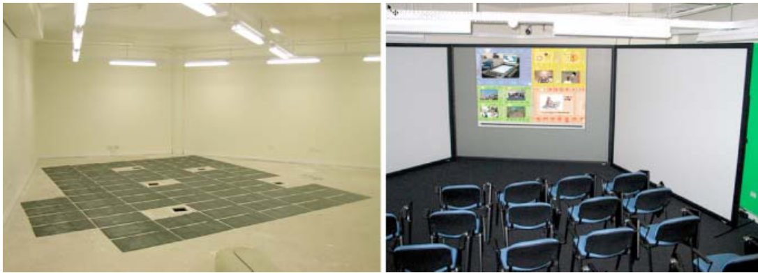
Fig. 6. The pressure sensitive pads placed underneath the carpet (left) and the Sentient with completed flooring (right). [A color version of this figure can be viewed online at www.journals.cambridge.org ]
