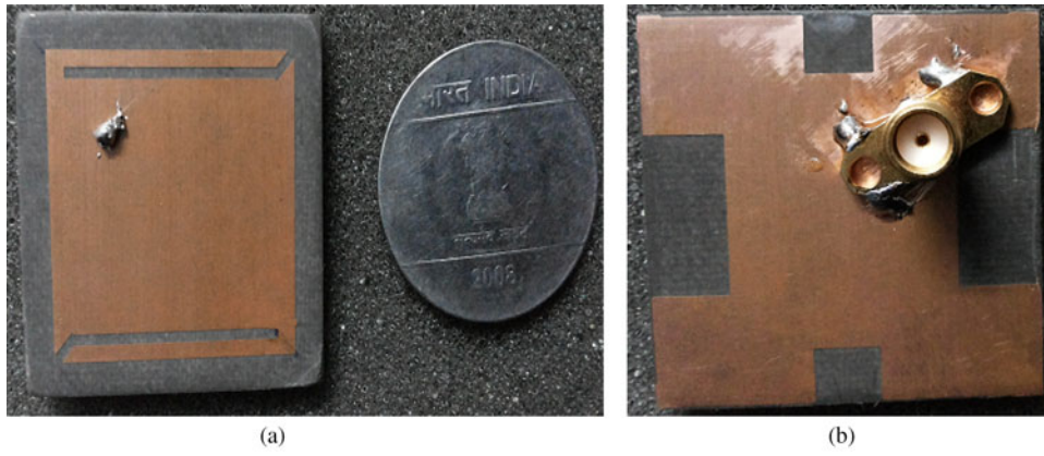
Fig. 7. Photograph of the proposed antenna working for L_1 and L_2 bands: (a) top view and (b) bottom view.
