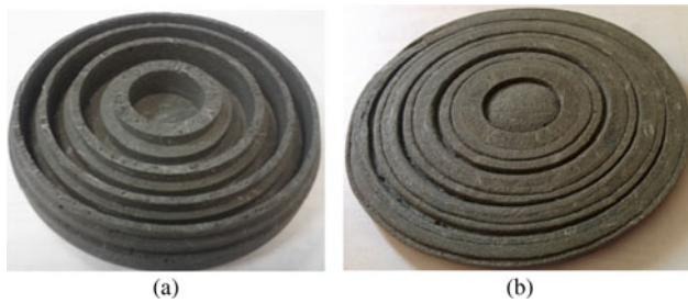
Fig. 3. FZPL4 ( q = 4 ) manufactured with the new technological process, (a) before being pressed, (b) after being pressed.
