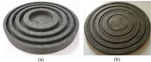
Fig. 2. FZPL ( q = 2 ) manufactured with the new technological process, (a) before being pressed, (b) after being pressed.
