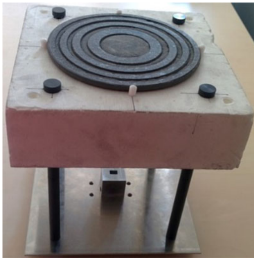
Fig. 4. Manufactured FZPL2 fed by the optimized horn antenna with foam support.
