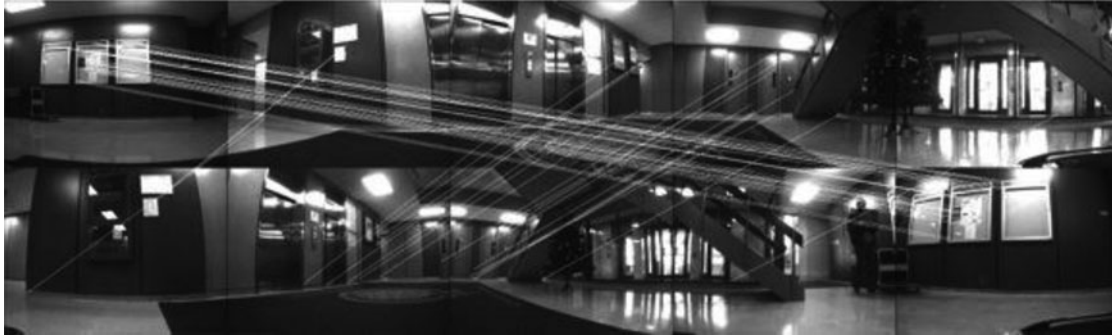
Fig. 4. A wide-field goal image (top) with SIFT features matched against a wide-field current image (bottom) using Lowe's SIFT tools. Matched features are connected with a straight line. Images are taken over a 270° pan.
