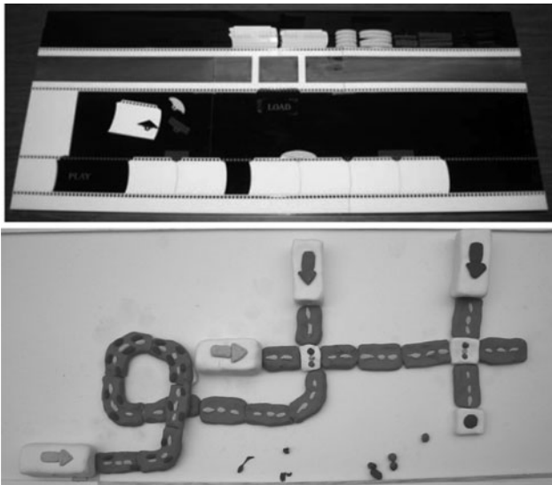
Fig. 5. Low-fidelity prototypes of (top) the TVE system and (bottom) the traffic flow simulator (from laser cut acrylic and modeling clay).
