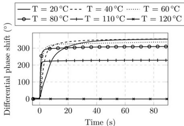
**Fig. 7.** Differential phase shift over time with different ambient temperature values up to the clearing point of the LC at 28 GHz with  $V_{bias}$  switched between  $-200$  and  $200$  V.
