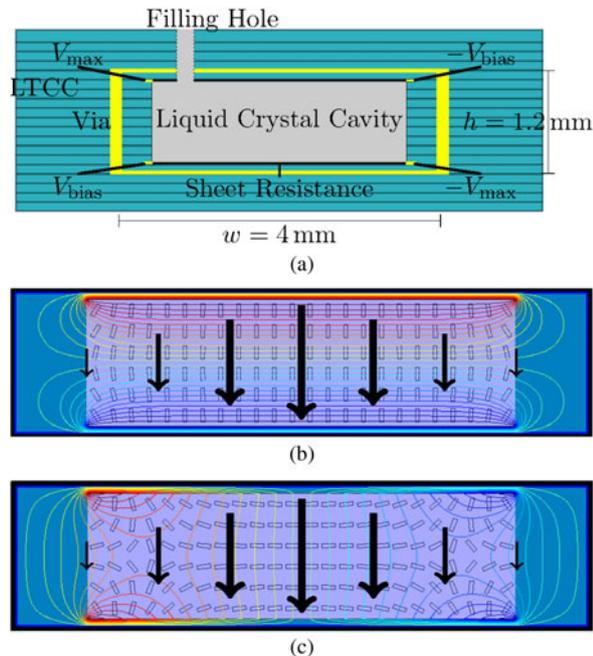
Fig. 5. Cross-section of the phase shifter with DC biasing field distributions and  $TE_{10}$ -mode.
