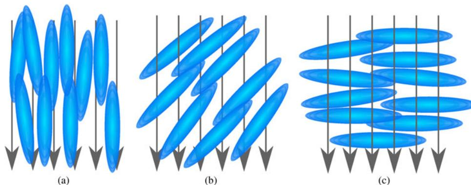
Fig. 1. LC molecule and the effective permittivities for the RF-field vectors.
