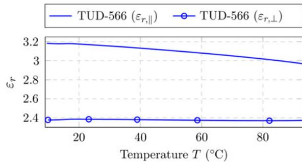
Fig. 2. Relative dielectric constant over temperature of the LC mixture TUD-566.
