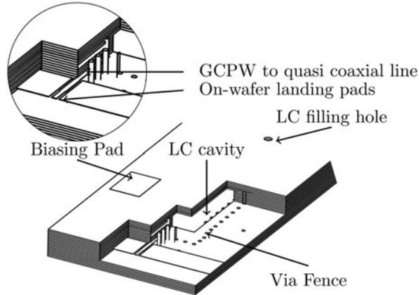
Fig. 4. Wire drawing of the transition part of the phase shifter test module.
