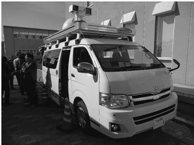
Figure 5a. A Small Satellite Ground Station.
