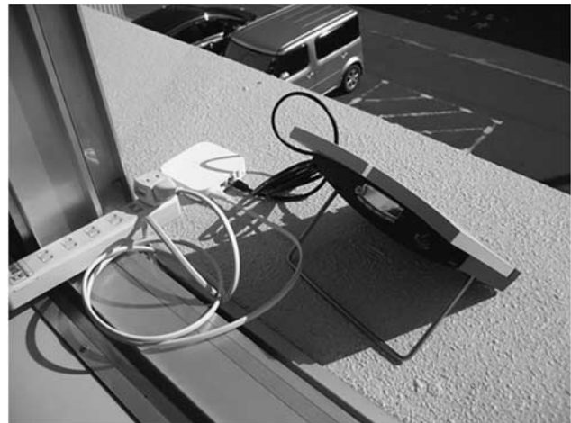
Figure 5b. A Satellite Communication Terminal for a Commercial Satellite Line (INMARSAT BGAN services).
