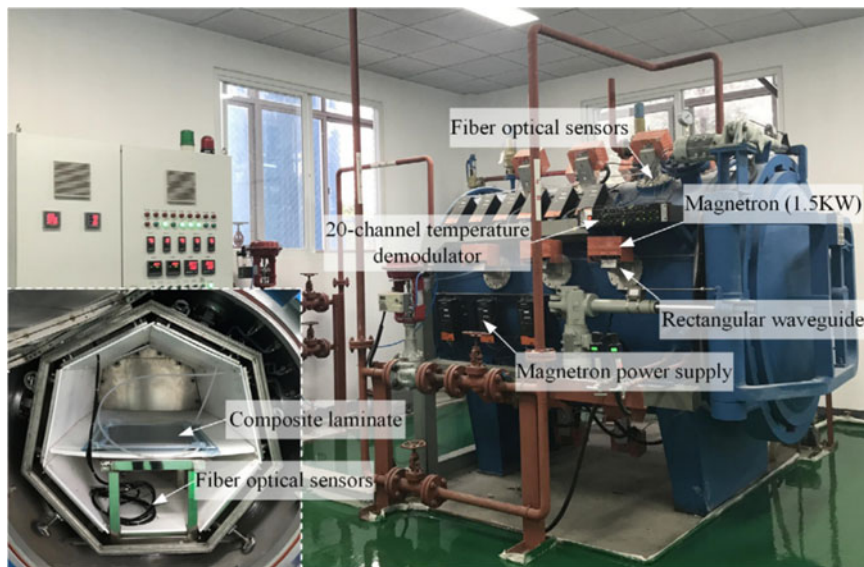
Figure 3. Photograph of the microwave curing equipment and optical fibre sensors used for temperature control (127) .
