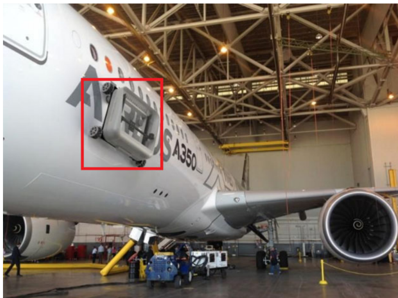
Figure 10. Photograph of the automated inspection platform (in the red box) attached on the cabin surface of an AIRBUS A350 (157) .
