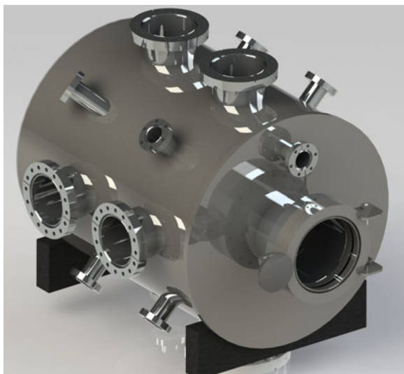
Fig. 3. 3D model of the space and planetary simulation chamber to be installed at AstroLab, without its accessories.
