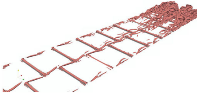
FIGURE 9. Contours of \lambda_2/\lambda_{2,min} = 0.0035 at the entrance of the non-periodic channel flow ( Re_b = 2093 ). Same range of x/h as in figure 6.
