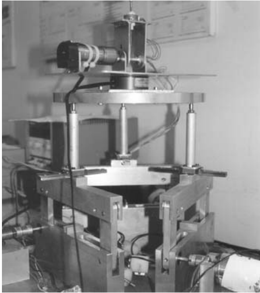
Fig. 1. The built prototype of CaHyMan (Cassino Hybrid Manipulator) at Laboratory of Robotics and Mechatronics in Cassino.
