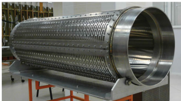
Fig. 3. Gas chamber of the XeF(C-A) amplifier with windows for electron beam injection.
