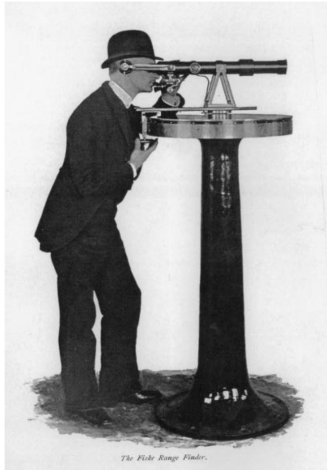
Figure 2. The Fiske Electric Rangefinder demonstrated by an engineer of the American Rangefinder Company (Anonymous, ca. 1895). Each of the two observation posts was mounted on a rigid stand. Each observer rotated his telescope to align on the target, thus changing the resistance in an integral electrical circuit contained in the cylindrical disc at the base of the telescope. A galvanometer at the gunfire control station read directly in yards. Note the telephone that could be used without the observer taking his eye from the target. Photograph courtesy Duke University Library, Perkins Pamphlet Collection.
