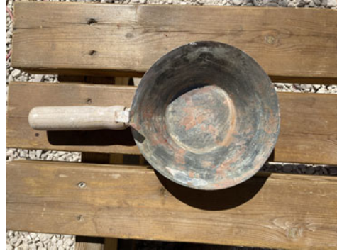
Figure 4. Builder's scoop (capacity: 0.7 l) used for our measurements.
