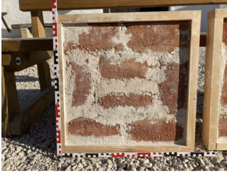
Figure 3. Framed bricks, onto which we applied our experimental mortars.
