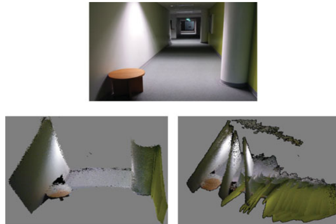
Fig. 1. (Top) A typical corridor in an office building with limited texture information. (Bottom) Alignment of multiple image using either (Left) only 3D features (Right) or only visual features. 19
