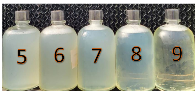
Figure 1. Visible observation of solubility of imazapic + nonionic surfactant at different carrier water pH levels.
