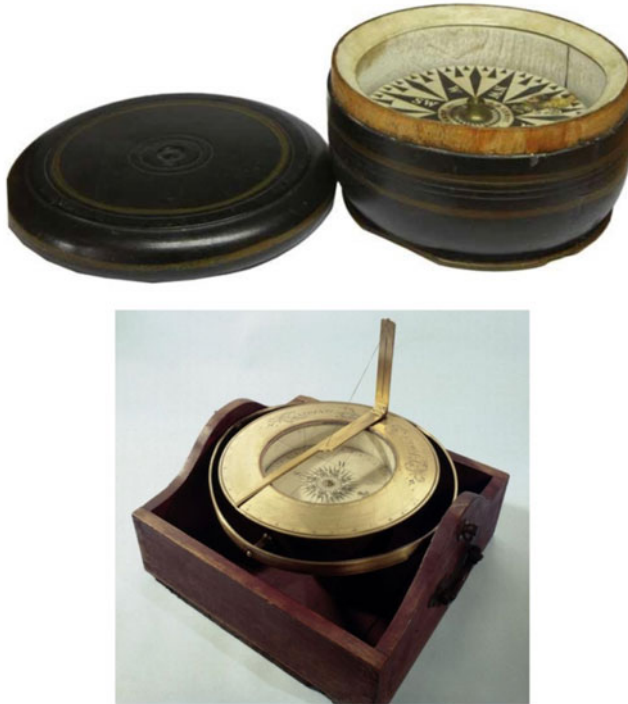
Figure 4. Wood-box Steering Compass, reproduced by permission of Paul Crespel. Brass Azimuth Compass © National Maritime Museum, Greenwich, London.
