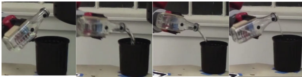
Fig. 16. An example execution of the pouring task for illustration. The four images show (a) the robot holding the bottle and waiting for the trigger to begin pouring, (b) the initial tilting phase where the liquid starts to rush out, (c) the middle pouring phase where the flow is more laminar, and (d) the untilting phase where the flow is cut off by the rising bottle edge.
