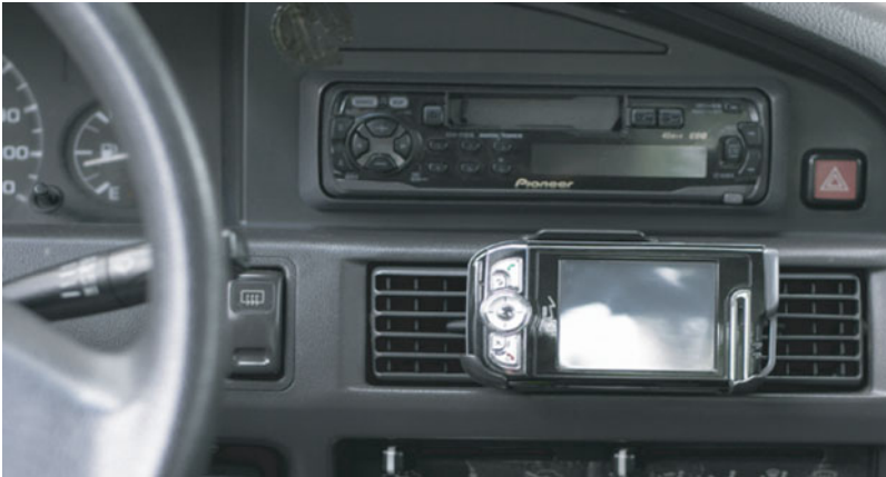
Figure 2. The PNS at the down position with horizontal (landscape) display mode.
