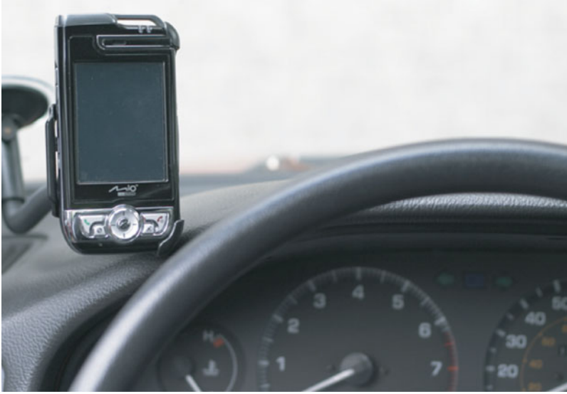
Figure 1. The PNS at the up position with vertical (portrait) display mode.
