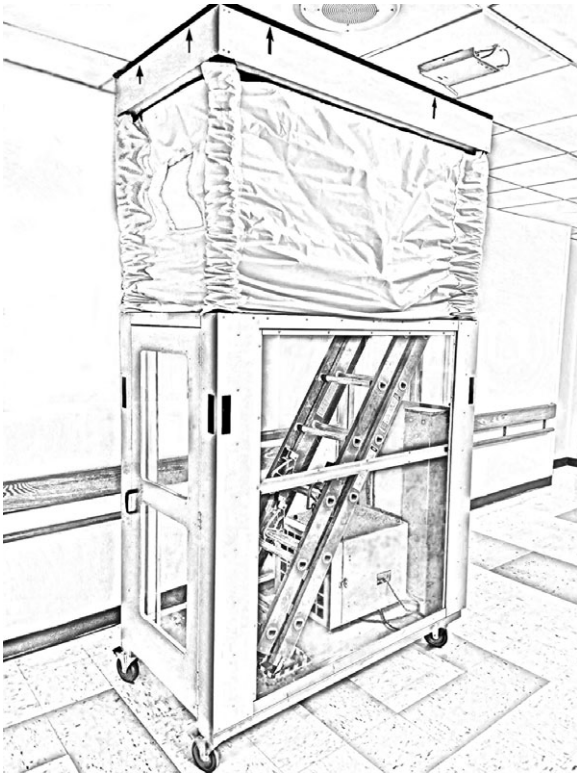
Fig. 1. Typical mobile dust-containment cart (MDCC) used for above-ceiling access.
